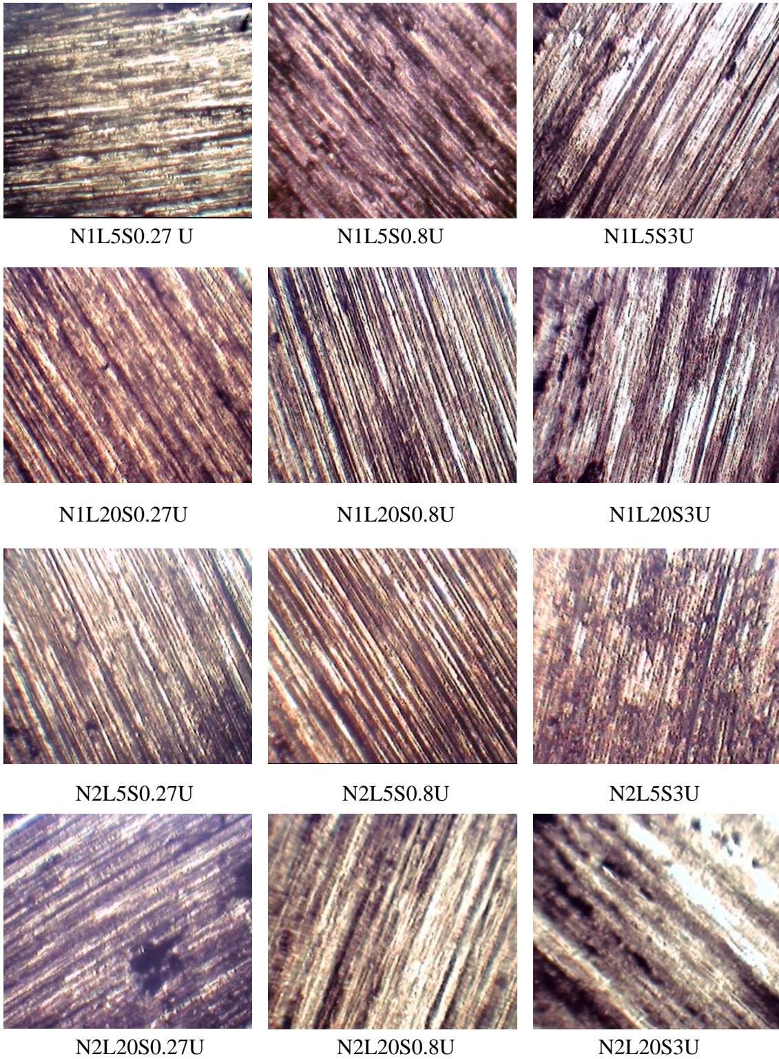
Fig. 75: Photomicrographs showing the shear lines at the worn ends after one hour running . ( N1: Al, N2: Al-Ti at Speeds = ( 0.27, 0.8, 3 ) m/sec and loads 5, 20 N)
