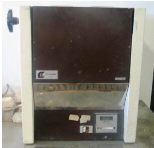
Fig. 13: Electric resistance furnace
